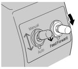
**12** Press  $\checkmark$  to feed some slack into the roll media.
